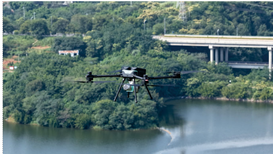
Sa130机载激光雷达巡查河堤
